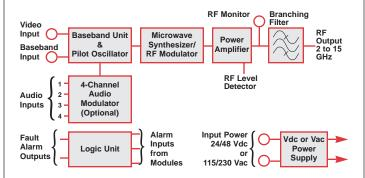
The FLR Series transmitter can be equipped with up to four optional audio modulators within the three-rack unit cabinet.
